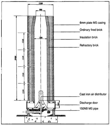
Figure 3: Technical detail of improved kiln design.
