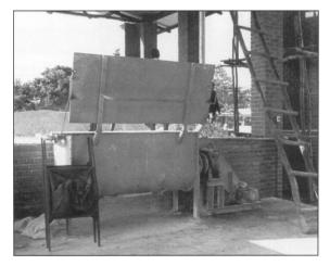
Figure 2: Prototype mechanical batch hydrator.
